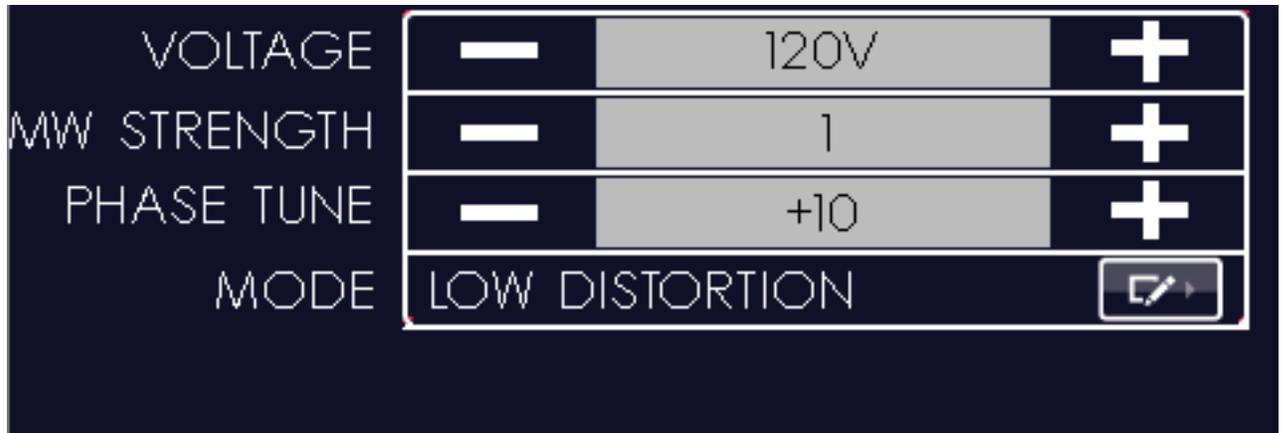
Each progressive step increases the charging time of the Power Plant's output waveform. Longer charging times, taking place at the peak of the Power Plant's output sine wave, lowers the connected equipment's power supply ripple, much the same way as increasing the power supply capacitance of connected equipment. Just imagine adding 50% more power supply capacitance to your connected equipment.
