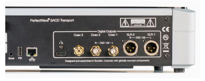
Although an HDMI cable is used for the I<sup>2</sup>S connections, it's important to note that I<sup>2</sup>S data is not HDMI data, and the PST's I<sup>2</sup>S output should not be connected to the HDMI input on a DAC or receiver. The HDMI connector and cabling are used only to deliver audio via I<sup>2</sup>S.
