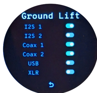
Figure 14: Ground Lift enabled on I2S 1, Coax 1 and Coax 2
