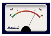
The Distortion In is a measure of the THD (Total Harmonic Distortion) present in your AC input voltage.
