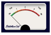
The Distortion Out is a measure of the THD (Total Harmonic Distortion) present in your AC Output voltage.
