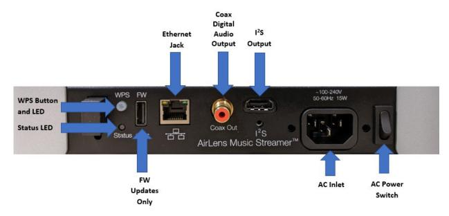
Connect PS Audio recommends connecting to your DAC through I<sup>2</sup>S protocol. I<sup>2</sup>S delivers the best sonic experience by separately transmitting data and clocks over an HDMI cable. A growing number of high-end audio DACs have adopted PS Audio's I<sup>2</sup>S standard, which we freely offer and support to the high-end audio manufacturing community.
